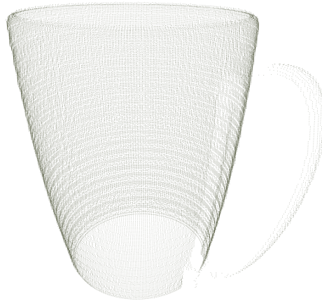
Figure 4.9: Point cloud of a coffee mug generated by the simulated scanner and related software.
