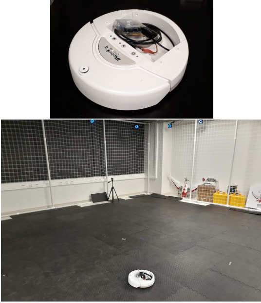
Figure 10: The iRobot ® Create ground vehicle with Odroid (top) and the experimental testbed with Mocap cameras at the RISC Lab (bottom).
