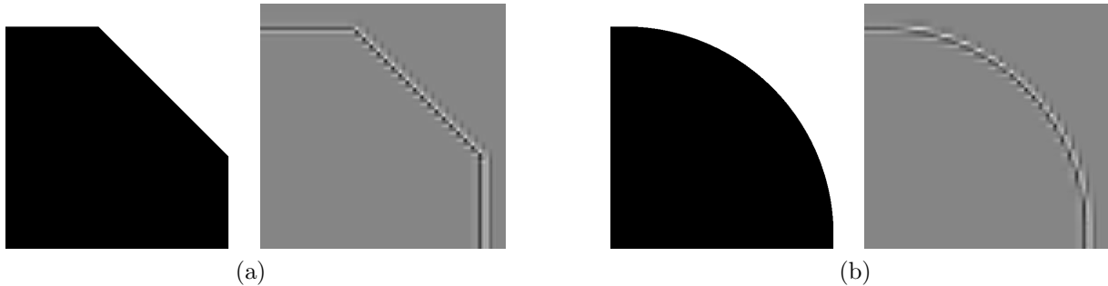
Figure 6.4: (a) Left: An image with three edge orientations. Right: Reconstruction of the image using only the fourth band Daubechies 2 wavelet coefficients. Note the irregularities on the edges that are not axis-aligned. (b) Same as (a), but using an image with a curved edge.
