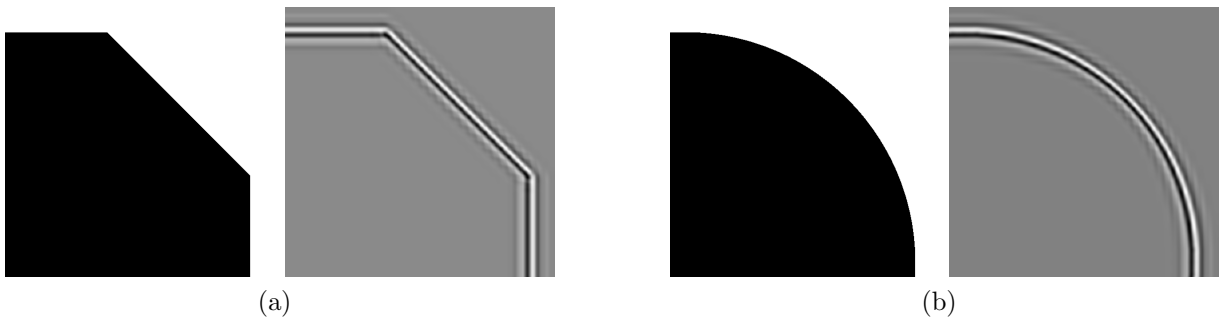
Figure 6.7: (a) Left: An image with three edge orientations. Right: Reconstruction of the image using only the fourth band DTCWT coefficients.
