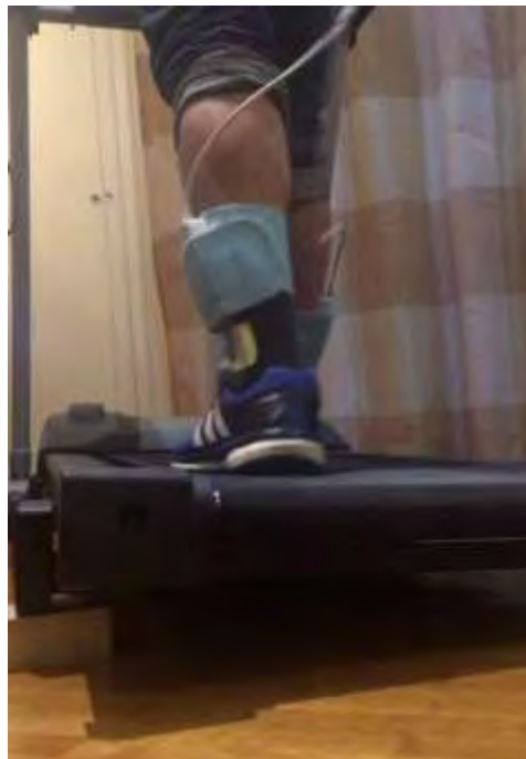
9: Plantar pressure measurement during inclined walking (4degrees left)
