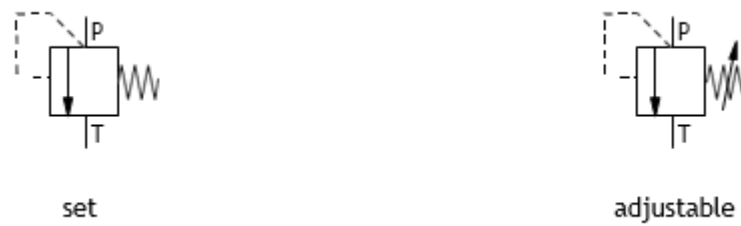
Figure 4-5 - Schematic of set and adjustable Pressure Valves. (D.Merkle, M.Thomes and B.Schrader. Hydraulics Basic Level Textbook )
