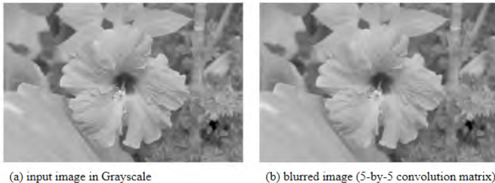
Figure 2.2: Gaussian convolution blur example with a 5-by-5 kernel which is used to Gaussian pyramid computation
