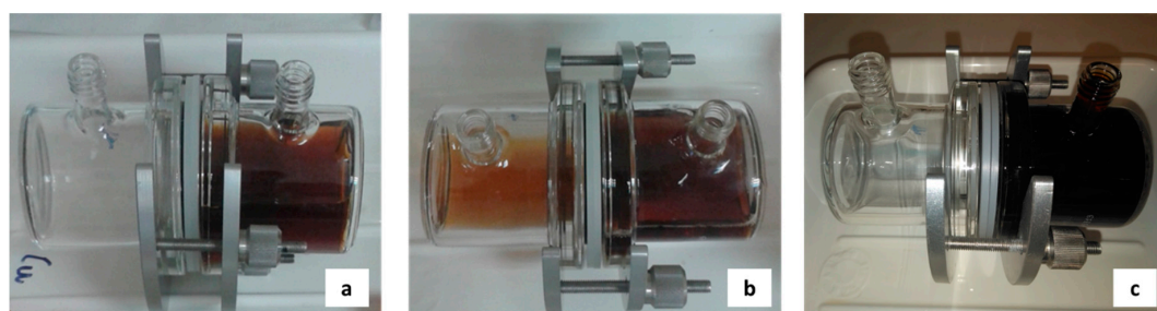
Figure 12. Images of the permeability tests of virgin PVDF membrane (a), SILM with CYPHOS 108 in PVDF (b), and SILM with [BMIM][DBP] in PTFE (c).
