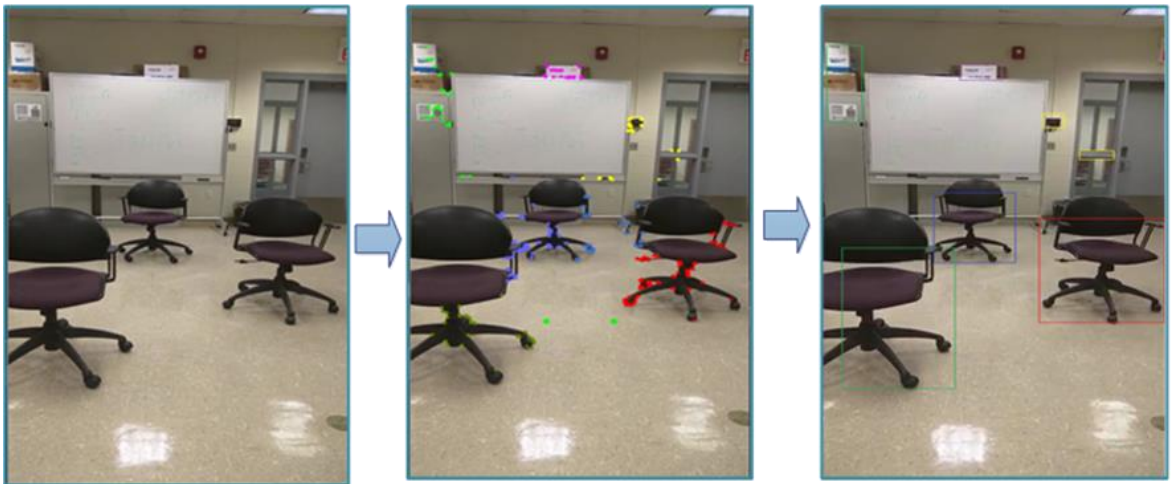
Figure 4. 6: Representation of the proposed object detection technique; (a) original frame, (b) the frame after applying proposed sequence of algorithms for object detection and (c) the frame after applying K-means clustering and merging to identify each object
