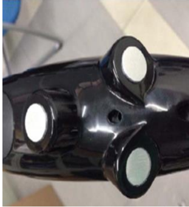
Figure 2.6: The replacement of the three ultrasonic sensors on the cane [24]
