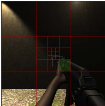
Figure 2: The VPR is more fine grained in the direction the gun is pointing. Shown is an example of the DCNN correctly predicting the class (green square) with a confidence of 55.7%, with only four pixels of the target being visible.
