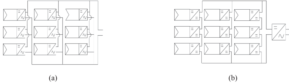
FIGURE 1. System layout based on microinverters (a) and serial DC power optimizers (b).
