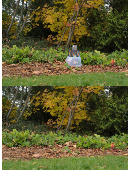
Figure 1. One image from each of the two bracketed sets for a single scene. The upper image includes the frame holding the 4 Gretag Macbeth mini Colorcheckers, the lower one right excludes it. The Colorcheckers on the top and sides are at 45 degrees with respect to the middle one.
