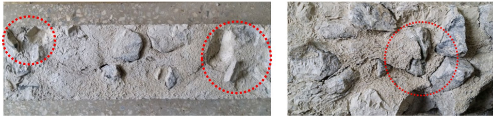
Fig. 3 Interfacial failure between recycled ballast aggregates and mortar in freezing–thawing tests (Yoo et al. 2016).
