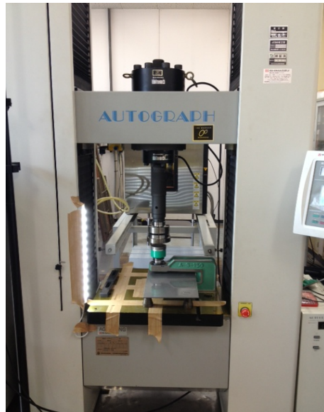
Fig. 3.5 The universal tension and compression testing machine which is used in the punching experiments.
