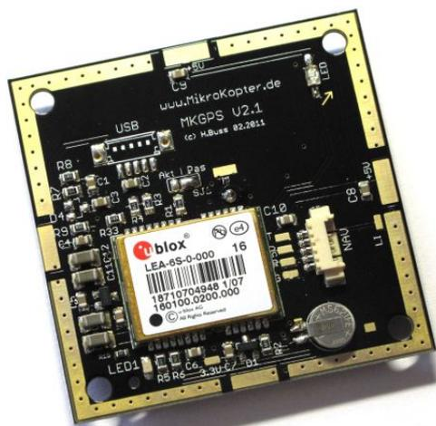
Figura 12. Receptor GPS MKGPS v2.1
