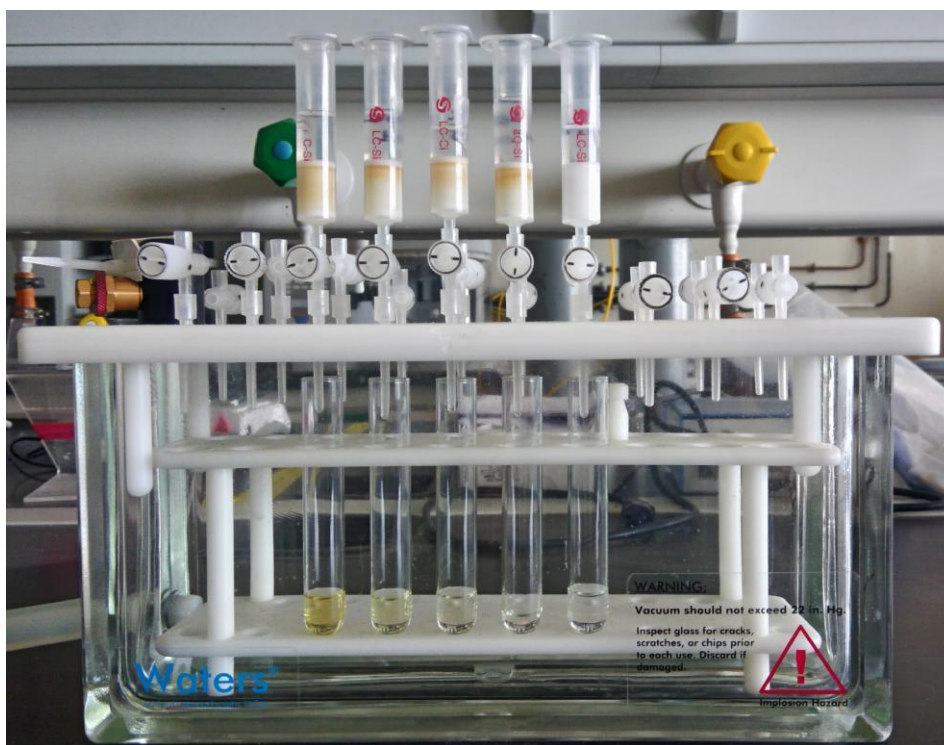
Fig. 2.8: Manual Solid Phase Extraction aspirated by vacuum with Silica columns while collecting the extract
