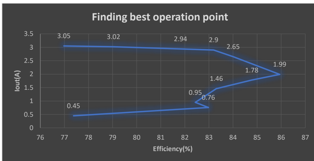
Figure 32 - Performance Graph for LM2596 Module
