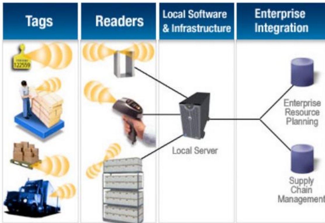
Figure 7- Working of RFID System.
