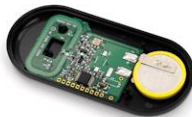
Figure 9 - RFID Active Tags. Semi-passive RFID
