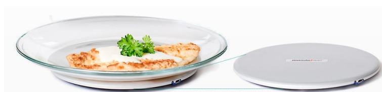
Figure 2. The Mandometer®, a device for continuous recording of eating behaviour in humans.
