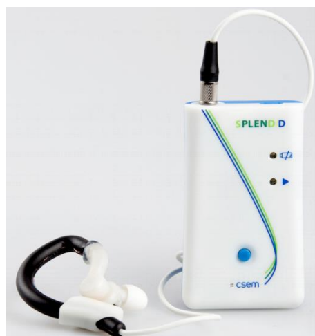
Figure 3. Device developed for use in detection of eating in the SPLendid EU project.
