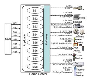
Figure 5: Design of integrated services using SCA
