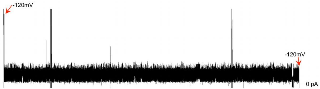
Figure 16. Continuous recording of the block by cross-linked mutant target/probe duplex E for 30 min at +120 mV, in 1M KCl, 10 mM Tris, pH 7.4 at 22 °C. The result demonstrates the permanent trapping and current blocking of the cross-linked DNA duplex in the nanopore.
