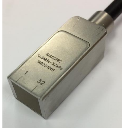
Figure 4.17. A photo of the transducer used in this study. The positions of the first and last transducer elements are marked. The linear array of transducer elements can be seen on the bottom.
