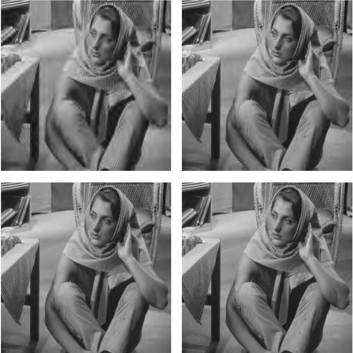
Figure 4.10 Comparison of Barbara image under different bitrate by SLCCA Plus. Top left: 0.1 bpp, 25.09 PSNR. Top right: 0.3 bpp, 29.82 PSNR. Bottom left: 0.5 bpp, 32.92 PSNR. Bottom right: 0.7 bpp, 35.32 PSNR.
