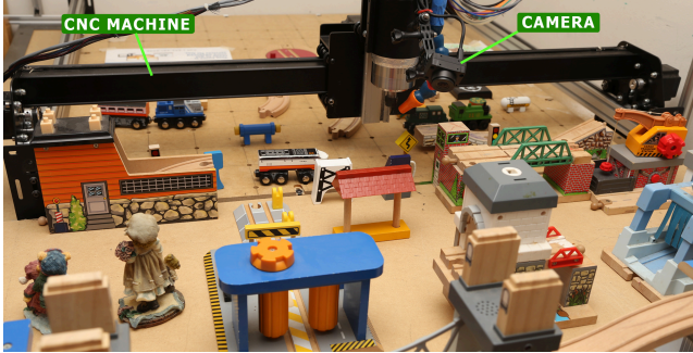
Fig. 8: Experimental setup showing a camera mounted on a CNC machine allowing us to capture ground truth information. Camera mounted on a CNC machine
