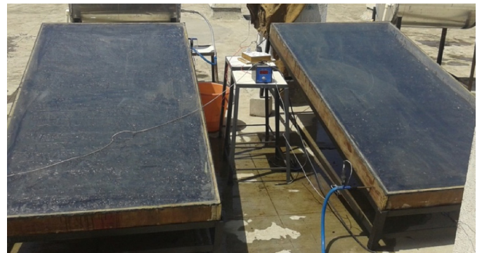
Fig. 7. Photo of simultaneous testing of dimpled tube and smooth tube concrete collectors.
