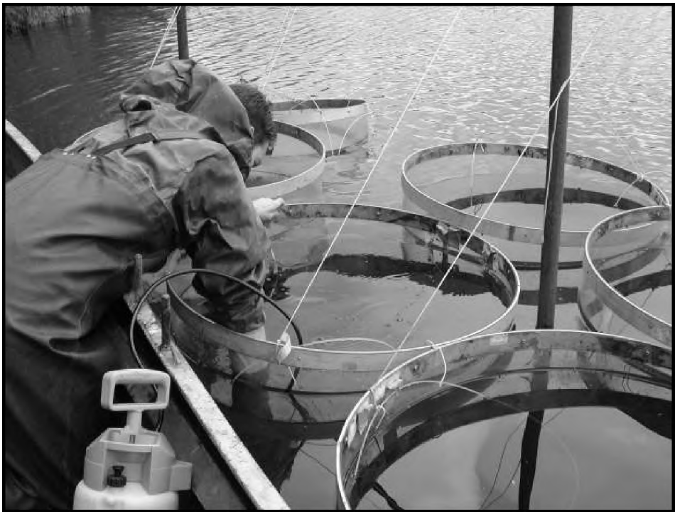
Injection of iron chloride solution into the sediment of enclosures in Lake Uddelermeer (The Netherlands; photo by Leon Lamers)
