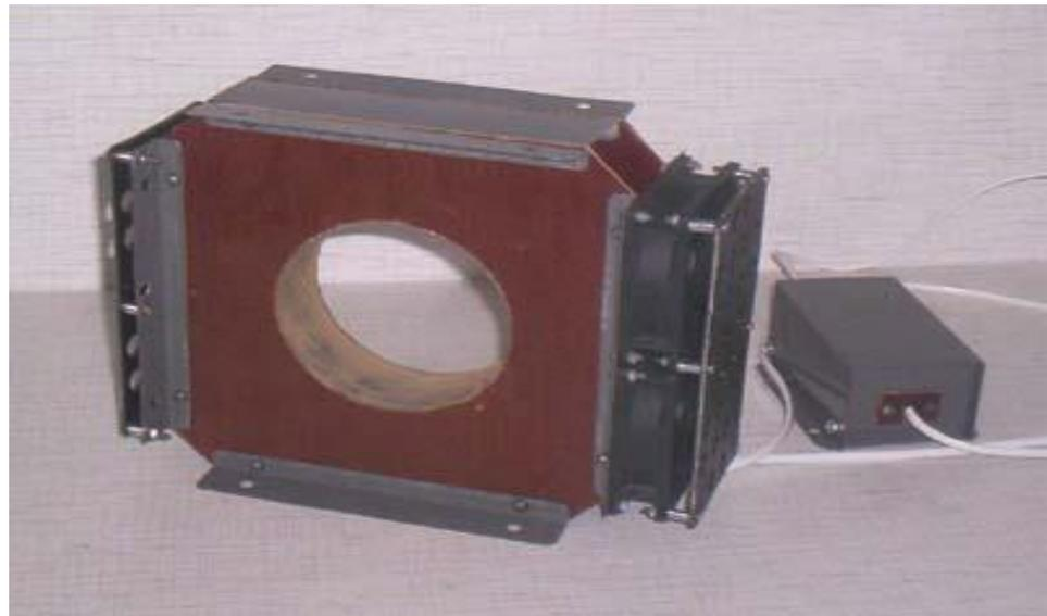
Figure 3 - Demagnetizer tunnel passage opening with a diameter of 100mm.
