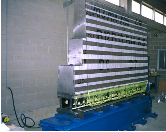
Figure 2.13: Section of the TileCal during assembling.
