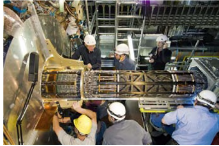
Figure 2.7: Installation of the pixel detector in ATLAS on June 2007.
