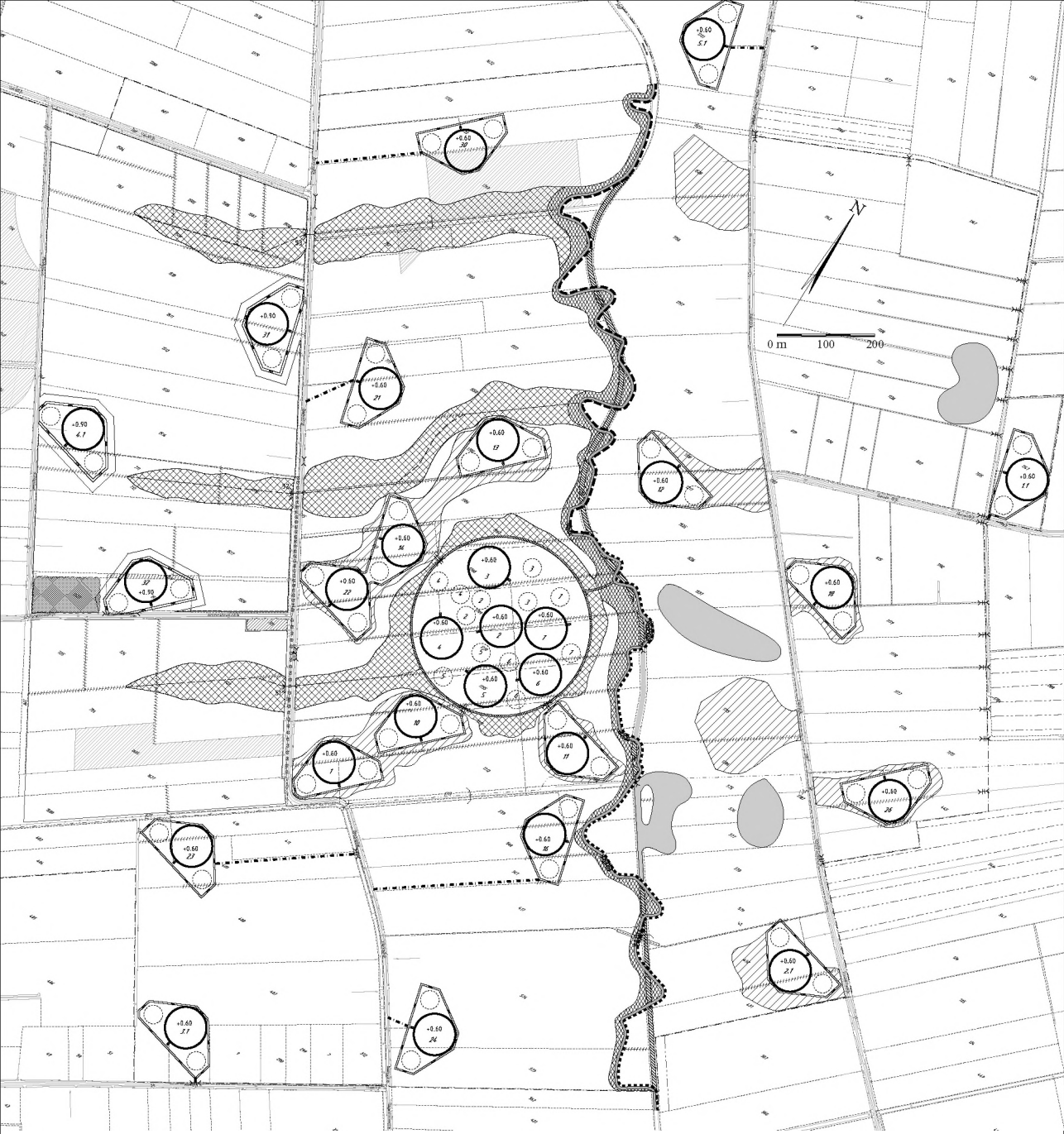
FIG. 6.1 · Overview of the station locations in LOFAR's compact core. Each station of 48 low-band antennas is indicated by a solid circle. Current funding allows construction of about half of these stations. (Drawing courtesy of Astron.)
