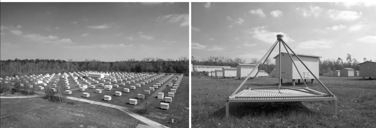
FIG. 1.3 · Overview of the KASCADE particle detector array (left) and one of the LOPES antennas (right) which were set up between the particle detectors.
