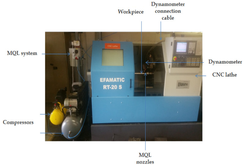
Fig 1. Experimental setup used for MQL assisted high speed machining of NiTi alloy.
