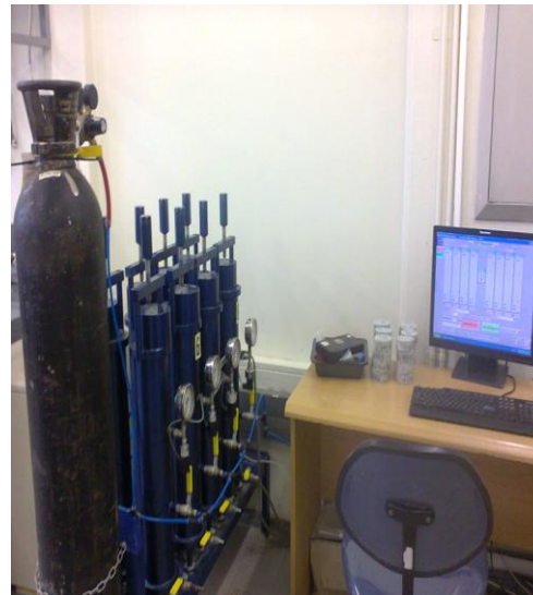
Fig. 1. Oxygen permeability apparatus setup used
