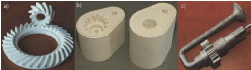
Figure 7. 3D printed gears (a) gear wheels, (b) gear wheel casting mould, (c) Al alloy casted gear made in the mould (Source: From [1], published under CC BY 4.0 license, available from: http://dx.doi.org/10.5772/22848 ).
