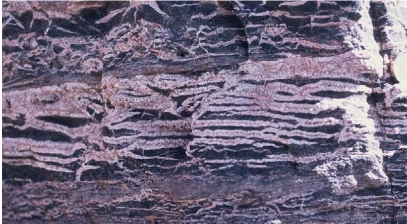
The clear, coarse-crystalline dolomite fill in veins created by hydraulic fracturing that tend to follow the original bedding of the rock
