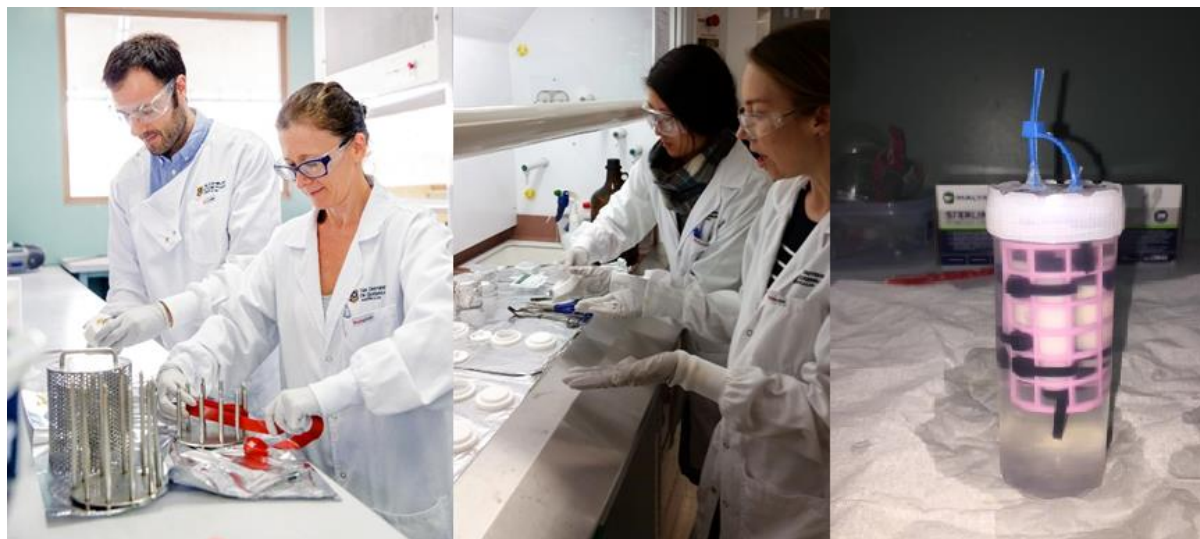
Figure 1. From left to right. Preparation of PDMS strip in stainless steel cage, preparation and assembly of ED samplers and deployment setup for a PE sampler.
