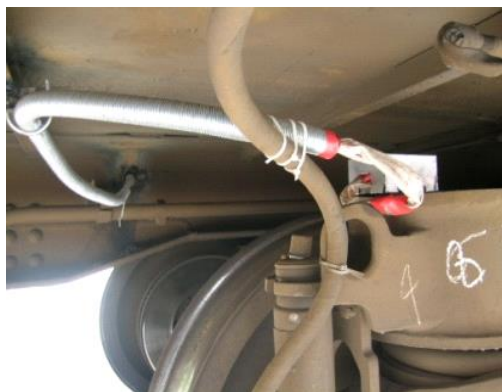
Fig. 2 Installation of the tri-axial accelerometer on the bogie frame
