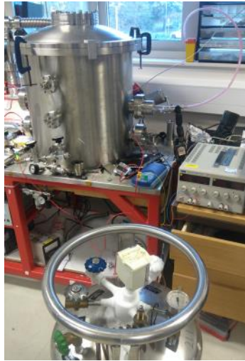
Figure 3 Thermal vacuum system
