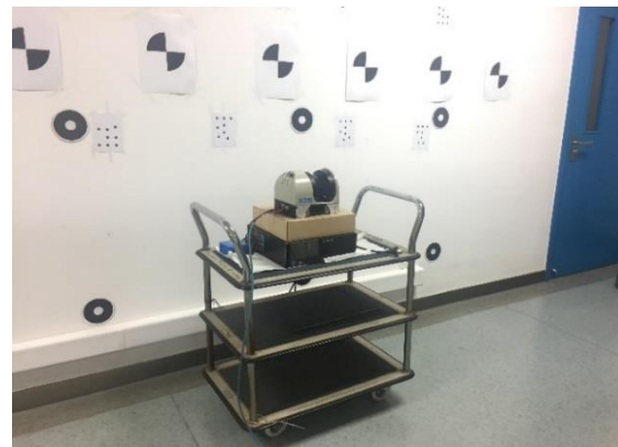
Figure 6. Laser scanner and IMU on a trolley
