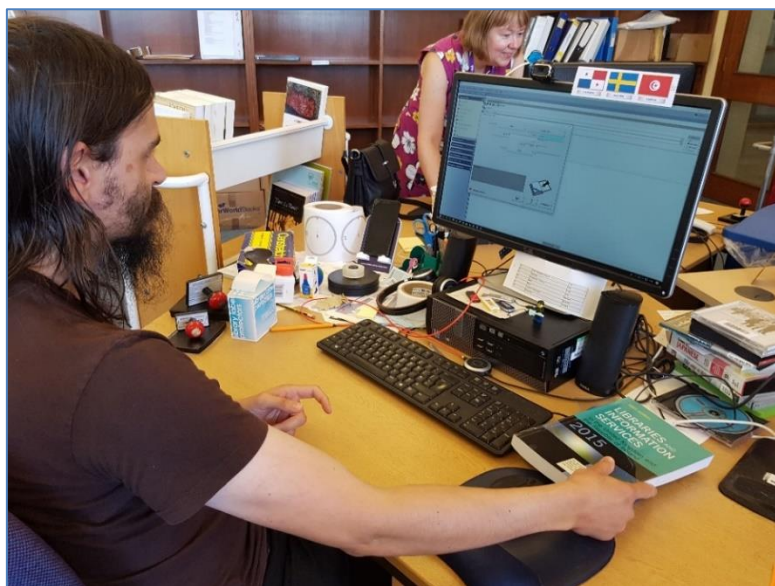
Figure 2: A member of the Collection Maintenance team using the RFID pad to check the tag of a book that has no barcode or process stamp in order to ascertain its barcode, and thus ultimately the identity of the book.
