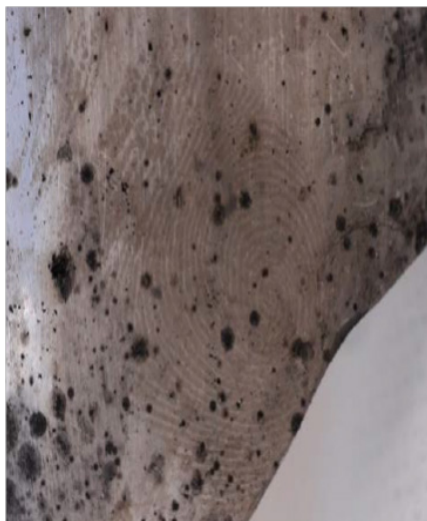
Figure 5 Fingerprint identified after soot removal with a soft brush. 39
