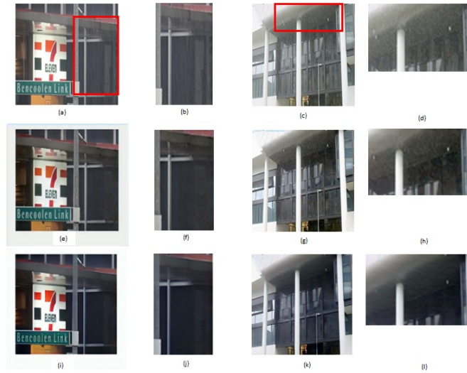
Fig. 2. Type I distortion for different severity of rain streaks as shown in Figure 2(a) to (d), and their rain removal results by the ID-CGAN and CycleGAN were shown in Figure 2(e) to (h) and 2(i) to (l) respectively.
