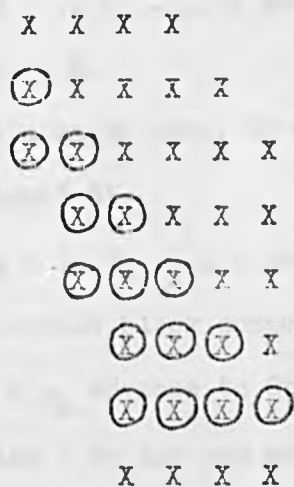
Fig. 2.13.1 The configuration at the start of the 8th major step in the LU factorization by stabilized elementary matrices of a stepped-banded matrix with q = 4 , p_1 = 3 , p_2 = 5 , p_3 \geq 8 .
