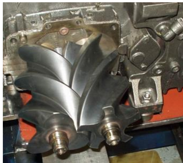
Fig. 8 Compressor rotors, housing removed
