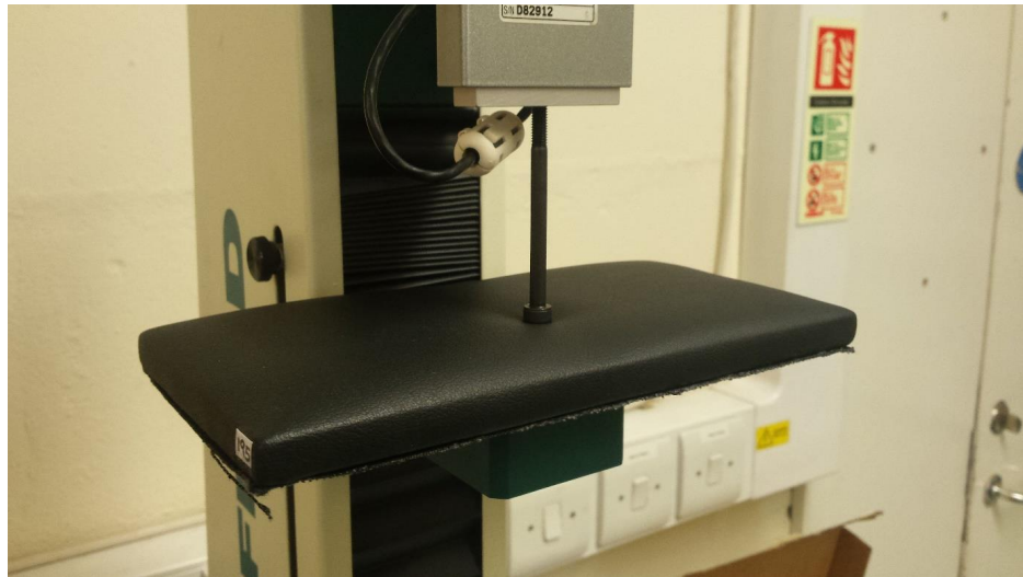
Figure 29: PVC Cuir grain (5mm) sample under a compressive load using the Hounsfield H1kS Benchtop Test Machine configuration. Source: Thompson (2016)
