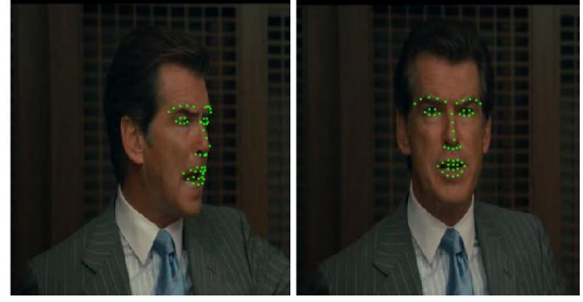
Fig. 2. Examples of detected facial landmark points and estimated head pose in terms of \theta_p , \theta_y , and \theta_r (best viewed in color).
