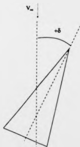
Figure 6.2. Definition of yaw angle sign. Delta wing viewed from above.
