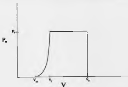
Figure 5.24. Wind turbine power versus windspeed.
