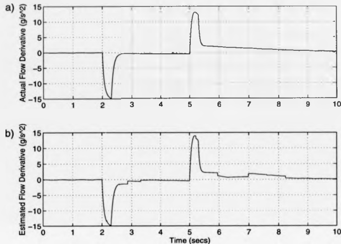
Figure 6.6: Actual and map estimated air flow derivatives for the simulation of figure 6.5.
