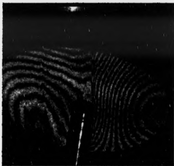
Figure 5.1: First holographic interferogram of vibrating board
