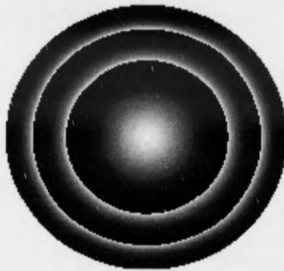
Figure 6.6: The wrapped phase map of the interferogram with M=3 (pixel samples in steps of 6 in y axis)
