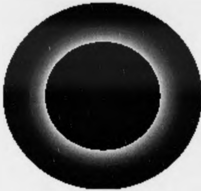
Figure 6.9: The wrapped phase map of the interferogram with M=1.5 (pixel samples in steps of 6 in y axis)
