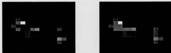
Figure 9.18: Square Sampled Five Item Input Image Together With Grey Level Morphologically Closed Version.
