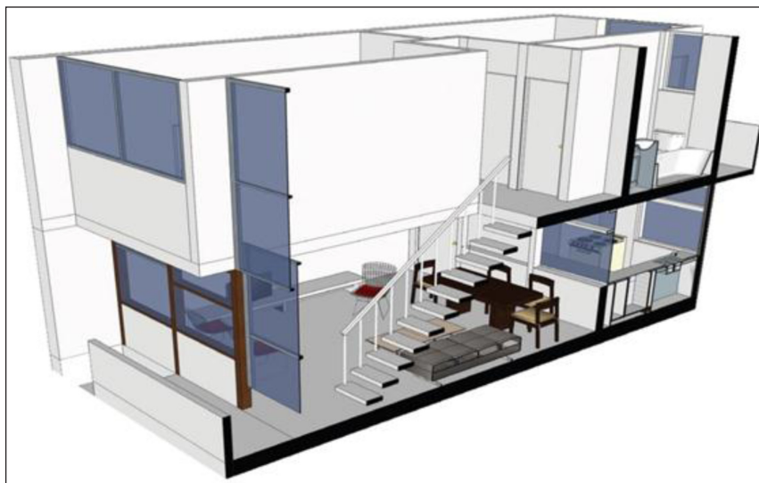
Figure 26: Axonometric view of a typical maisonette in Bayer House.
