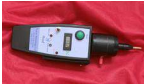
Figure 5. Image of the PRoD algometer (Topcat Metrology®)
