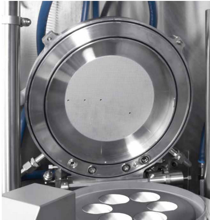
Figure 2.15: Showerhead of a MOCVD reactor [Aixtron SE]. At the bottom the susceptor with loaded wafers can be seen.
