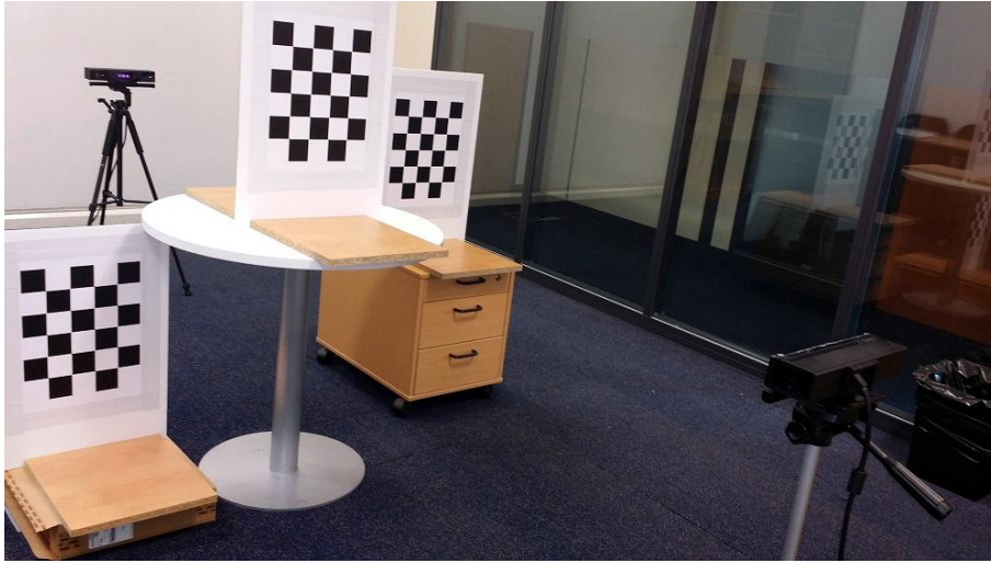
Figure 5.2: Two facing Kinects are placed at a distance of \sim 3\text{m} from each other which provides sufficient space for the data acquisition. The optimal location for minimal depth measurement noise is in the middle of the two Kinects according to our study in Chapter 3. Three double-sided calibration chessboards are placed at different depths to provide more distinct correspondences over the whole calibration space.
