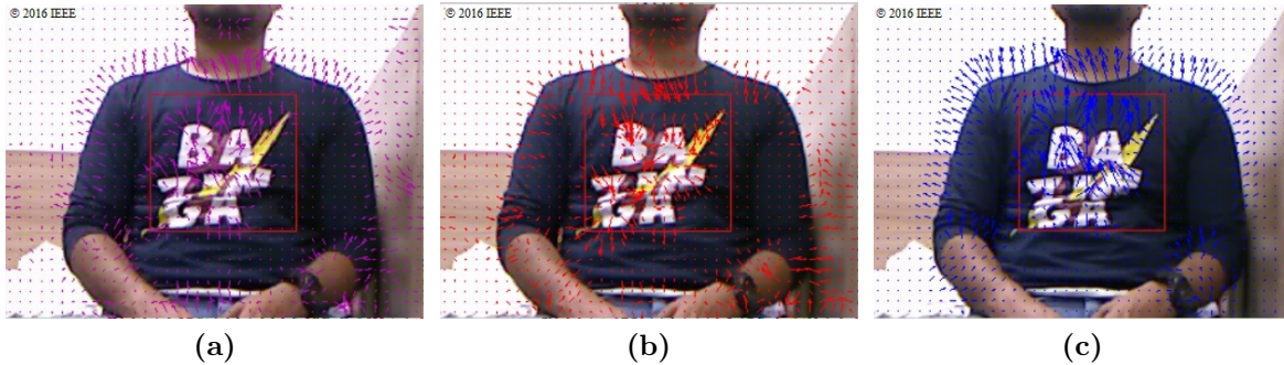
Figure 2.3: (a) Inhalation and (b) exhalation visualisation of flow field. (c) Visualisation of PFF . Images are taken from [50].
