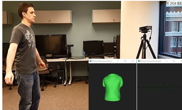
Figure 2.5: Subject’s standing posture during respiration monitoring [192]. Participants are constrained to keep up their arms away from the trunk to avoid occluding the chest-wall lateral sides. Images are taken from [10, 192].
