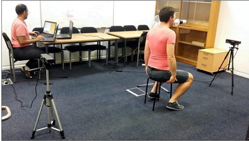
Figure 3.4: Data acquisition setup for collecting the depth-based PFT dataset using two opposing Kinects.
