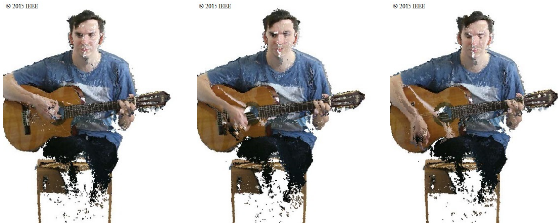
Figure 2.2: 3-D reconstructed models of a subject playing guitar using 4 Kinects by Kowalski et al. [106]. Spatial registration errors are observable especially on the face, hands and fingers which have more visual details. Also legs 3-D data has not been captured even by using 4 Kinects. Images are taken from [106].
